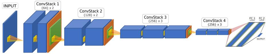
**Fig. 1.** VGG-12 architecture: blue, yellow, orange, and green are activation, convolution, max-pooling, and drop-out layers, respectively. Each number in the bracket reflects the depth of the corresponding convolutional layer.
